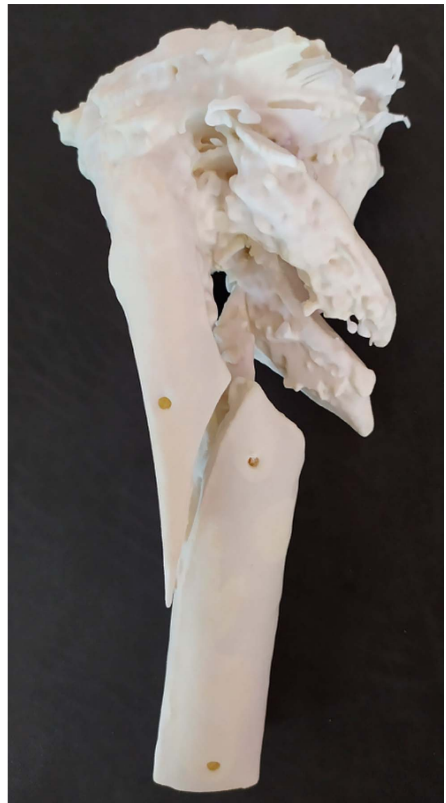
3D plastic printed part made according to the scanner of the right tibia
